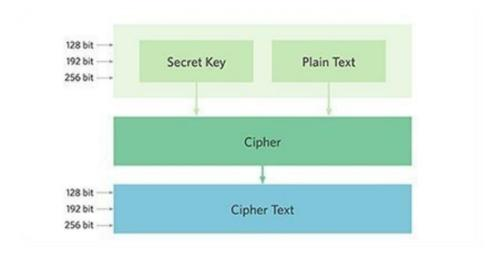
The schematic representation of AES Encryption
