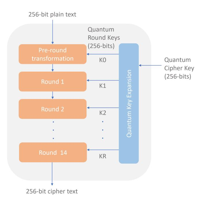
Here the Quantum Cipher Key is generated from a Quantum Random Number Generator which ensures true randomness and makes it secured from best possible known attacks.
